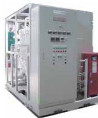
Ethanol / IPA Recycle System Package (Type:HDS-100)
