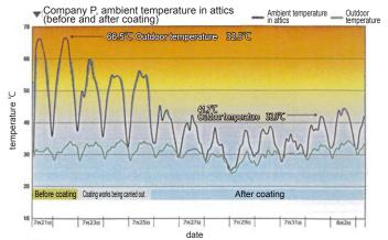
Roof coating with the insulating paint, combined with previously implemented energy-saving measures, further reduced CO2 emission by 22 t/year and the power consumed by air conditioning by approximately 9% (actual measured values).
