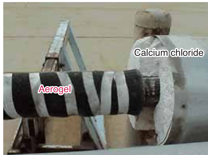
Photograph of Comparison in Thickness between Materials Same in Heat Insulation Effect
