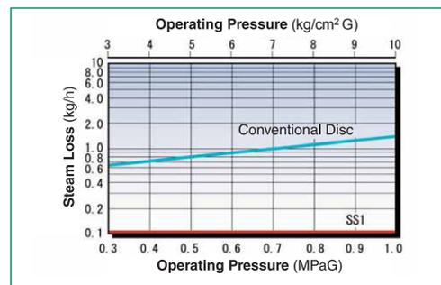
Steam Loss (Condensate Load: 5 kg/h)
