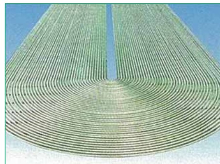
External appearance of heat transfer tubes for steam generator
