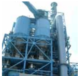
SNCR denitration equipment (Urea solution system)
