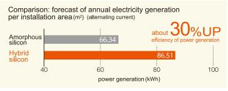
A case of low angle (5 degrees) installation, due south. 'Osaka-city. A case of low angle (5 degrees) Based on Kaneka's power generation forecas
